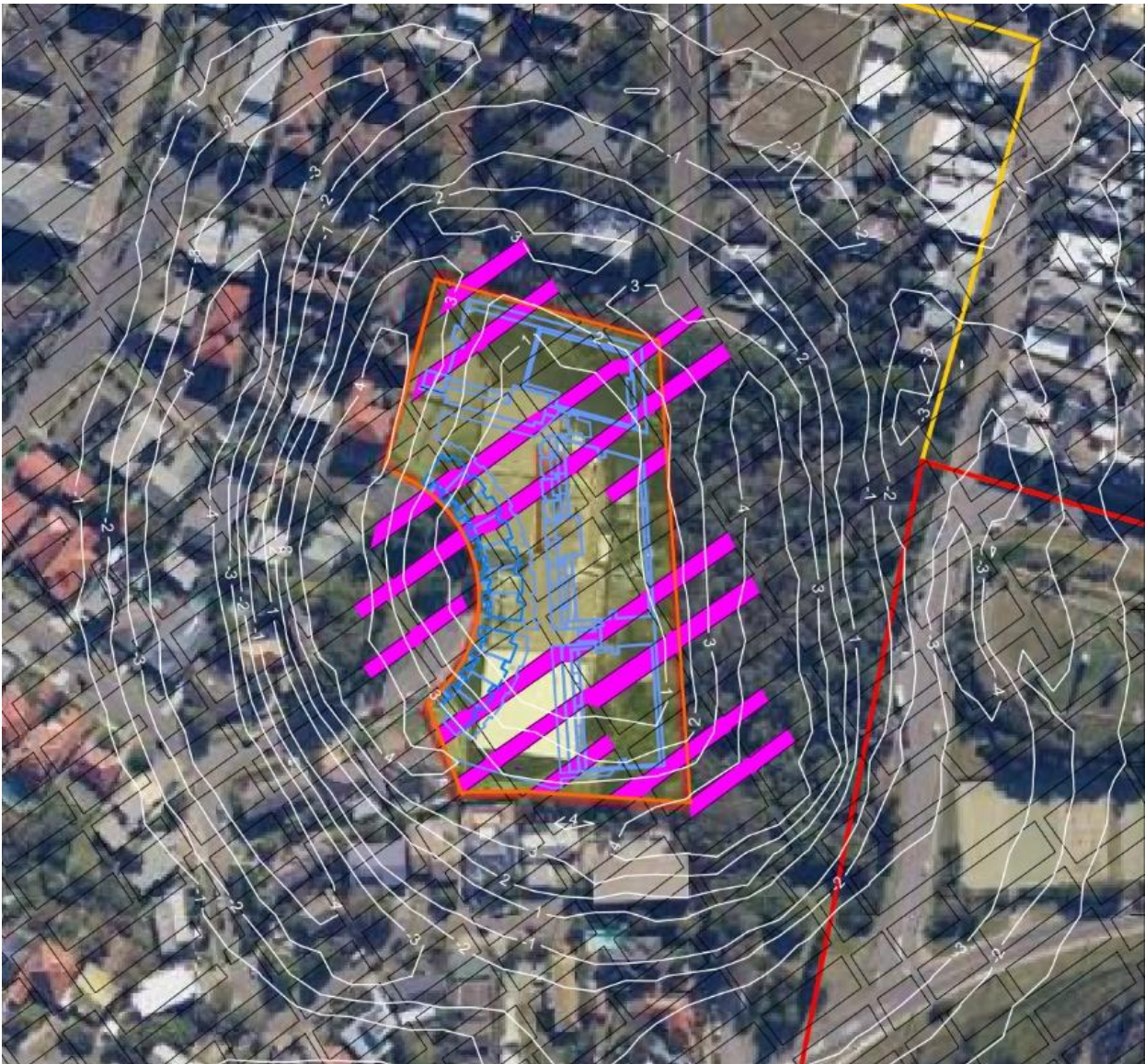
Fig 4: Predicted Final Horizontal Strain Contours with Aerial Photo and Proposed Grout in the Borehole Seam: Preferred Option 2 prepared by Ditton Geotechnical Services
