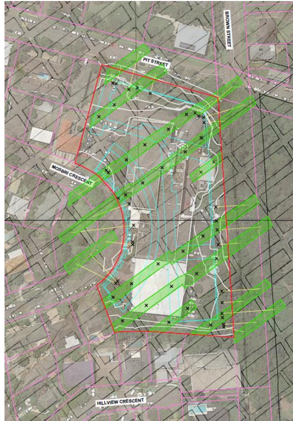
FIG 2: Borehole location for grouting the Borehole Seam.
